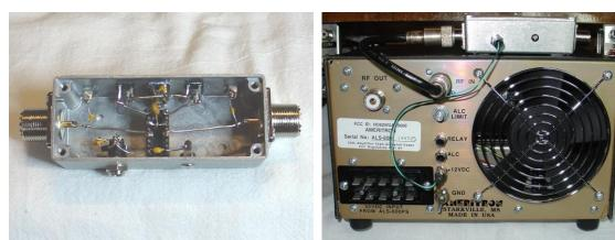
Photo E: 2dB attenuator inside view
